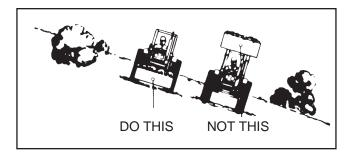
When transporting the load, keep the bucket as low as possible to avoid tipping, in case a wheel drops in a rut.
